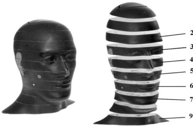
**Figure 1.** Head/neck region of an adult Rando phantom. Numbered slices indicate the levels containing thermoluminescent dosimeters.
